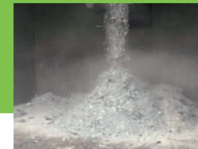
**We process the collected hardened thermoset composite parts and production waste through our recycling method.**
